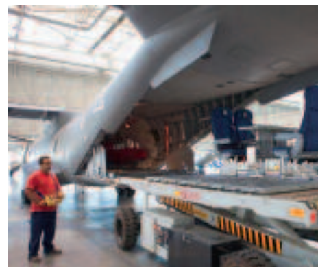
Highly versatile: Pallets are loaded through the rear ramp of the aircraft, enabling numerous configurations.
