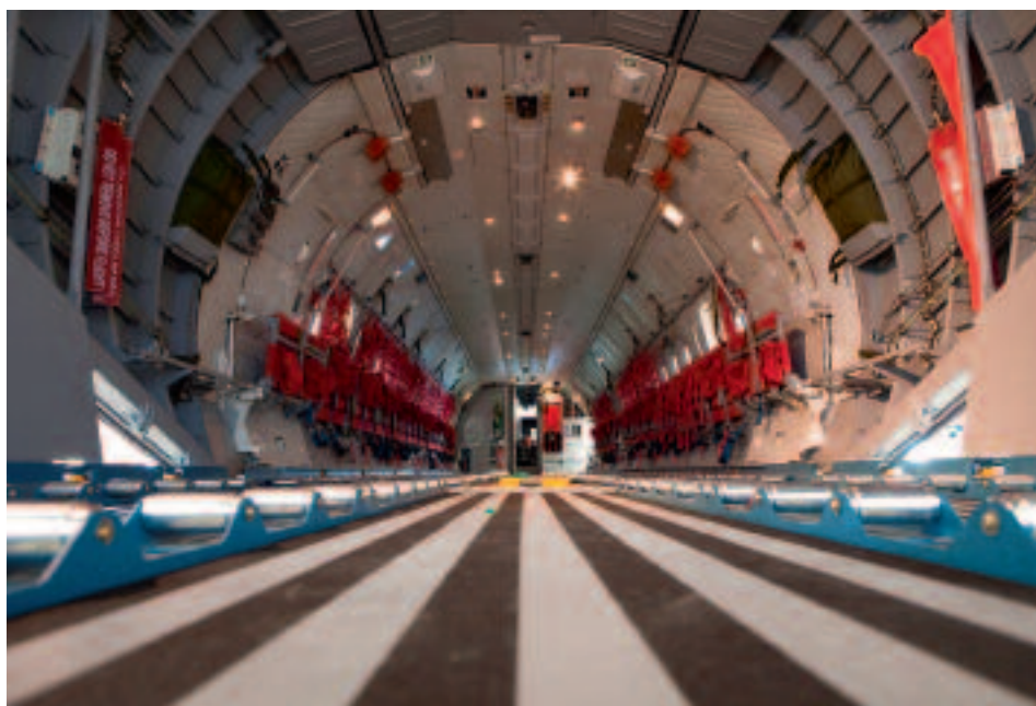
A cargo handling system guides pallets into position in the cabin where they are blocked manually.
